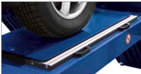
Precision sliding plate Minimal break-off torque 5 Nm and minimal push force 15 N, collection grooves for waste water.
