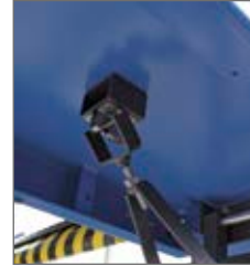
Fastening system and locking device for runway support.
