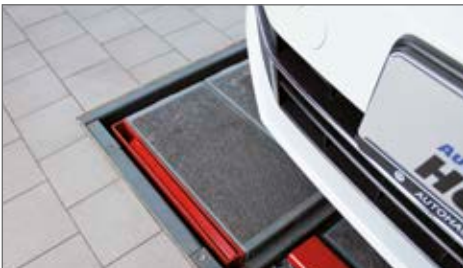
The floor compensation under the runway is a second ground surface, which levels off the surface below the lift.
