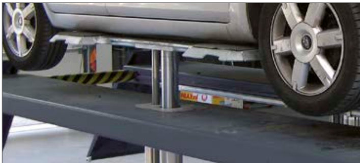
Runway lifts with flat head wheel-free jack, sill supports, load cap. 3.5 t
