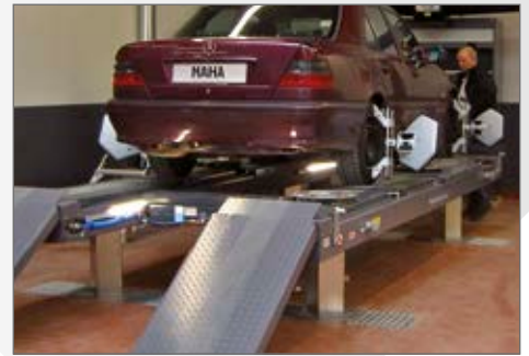
Highly accurate as a wheel alignment lift
