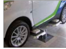
Shortened flat head support, for example 1150 – 1750 mm for the Smart
