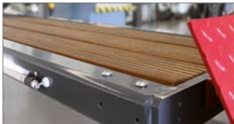
Runways with wooden covering for durable wheel tread and cutting edge design
