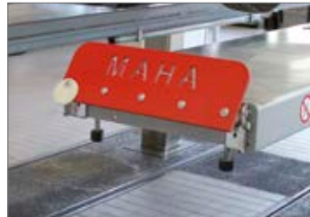
Automatic folding roll-off protection
