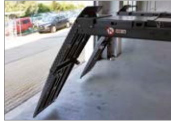
Folding drive-on ramp for high runways or low drive-on angle
