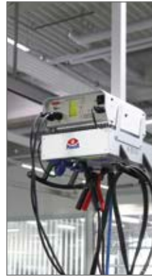
E-BOX with DEUTRONIK charging computer
