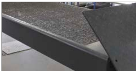
Powder coating with granular wheel contact surface
