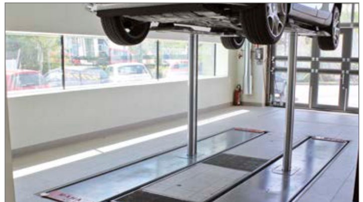
Vehicle lifted by the sill
