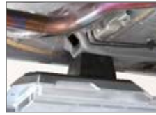
Pyramid block for highly accurate support and high freedom of movement under the vehicle
