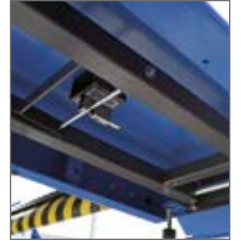
Fastening system and locking device for runway support.
